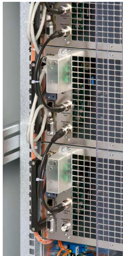
Closeup of Share bus and master-slave bus
